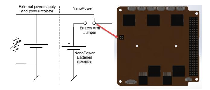
Example: With a voltage of 7.4 V and a 5  $\Omega$  resistor the simulated battery can sink 7.4 V/5  $\Omega$  = 1.48 A of current and the resistor must be able to dissipate 7.4 V \* 1.48 A = 10.9 W.
