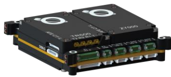
SDR MK3 NanoCom Link S TR600 Slot A ↔ ANT2150-DUP Slot B and C Empty
