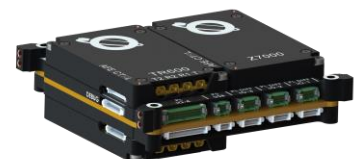
SDR MK3 NanoCom Link SX TR600 Slot A ↔ ANT2150-DUP TR600 Slot B ↔ ANT8250 Slot C Empty
