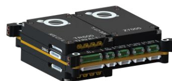
SDR MK3 NanoCom Link SX TR600 Slot A ↔ ANT2150-DUP TR600 Slot B ↔ ANT8250 Slot C Empty
