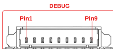
Figure 9.12: Debug and programming pinout
