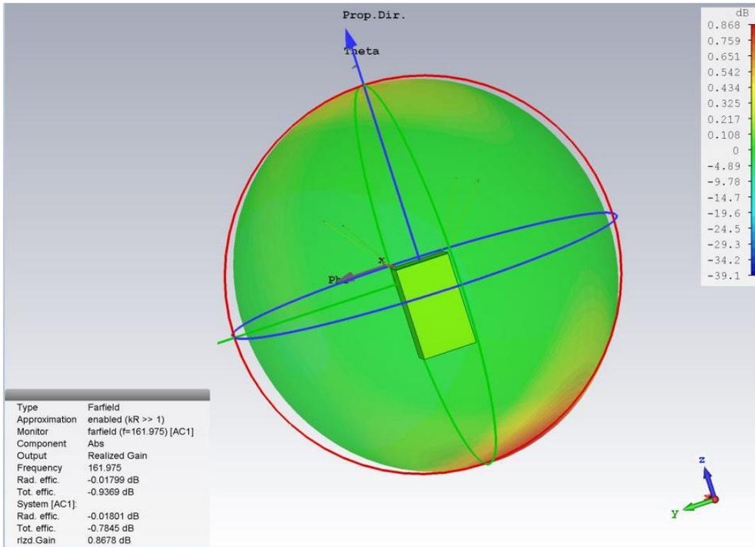
**Figure 13 Farfield realized gain simulated by CST program. The illustration shown in 3D view, including the satellite orientation.**
