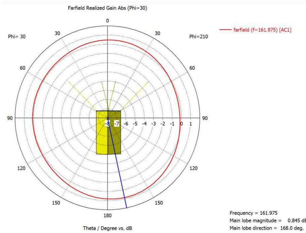
**Figure 12 Farfield realized gain simulated by CST program. The illustration shown in polar coordinate looking 30° into the 3U side of the satellite, including the satellite.**
