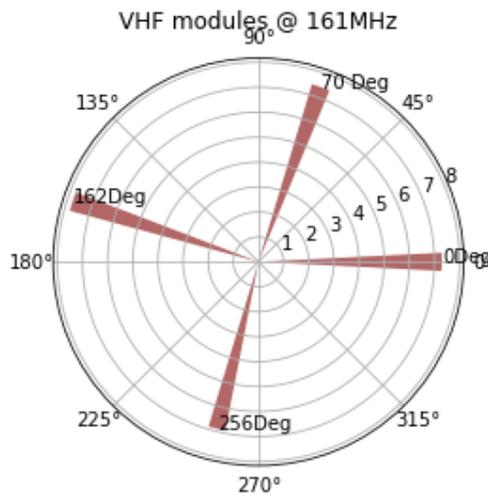
**Figure 11** Phase illustration in degree in polar coordinate in terms of relative amplitude in -dB at 161 MHz. The reference channel is channel 2, which set to zero. Channel 1, 3, and 4 are represented clockwise, respectively.
