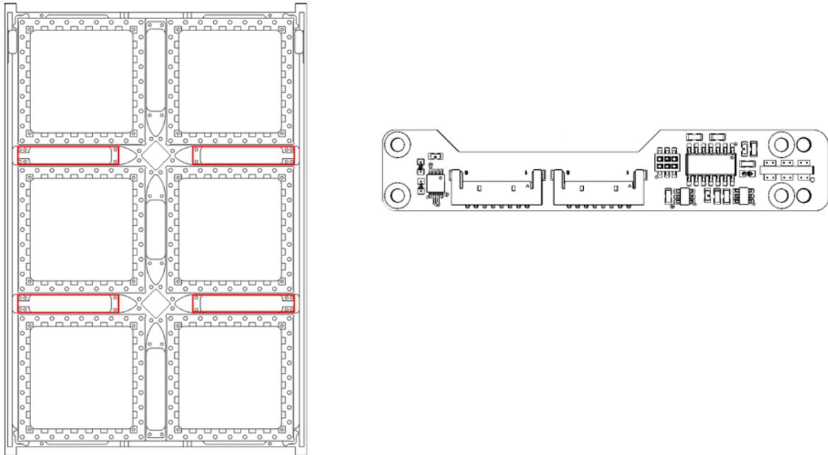
The front of the PCB contains all the electronics and connectors. The bottoms only contain the countersunk holes for mounting. Except for the antenna release, the whole PCB will be covered from the outside by solar panels.
