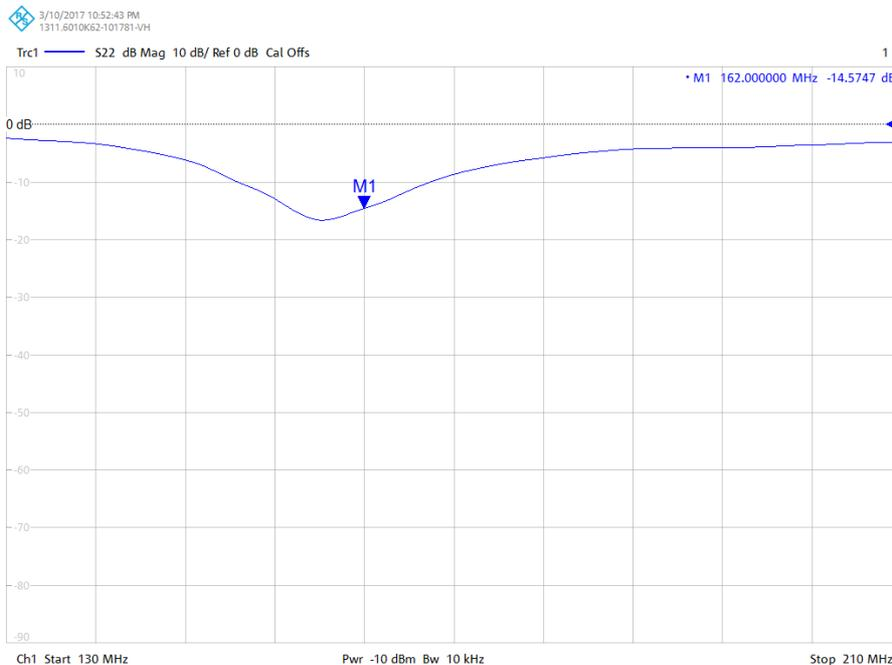
**Figure 15** Return loss of one of the antenna ports with antenna rods and with matching components mounted on the other ports. Also, the full system installed on a 6U structure for more realistic results.
