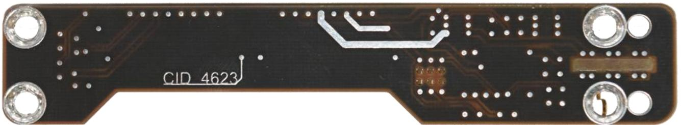
Contains no components. Four countersunk holes for M2 screws.
