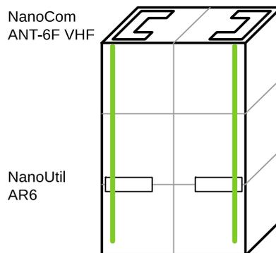
**Figure 6 6U structure with mounted ANT-6F VHF on the top and AR6 on the side. Antenna rods (in green) stowed down the side**
