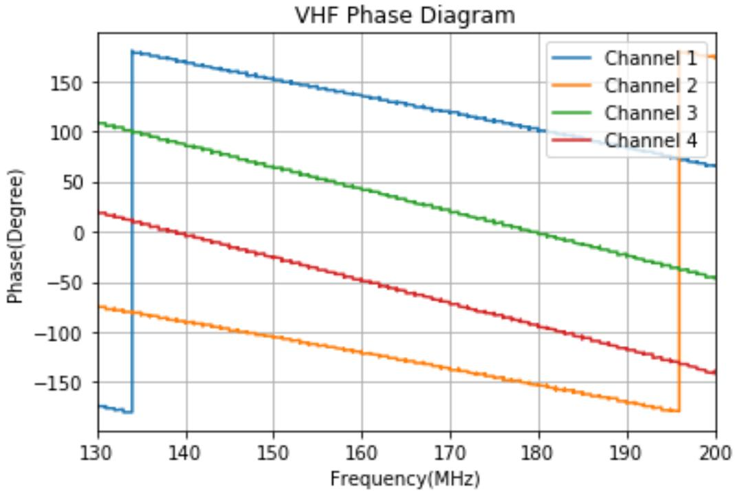
**Figure 10** Signal has been sent at Input 1 and each color corresponds to the measured signal at different channels / U.FL antenna connectors. This is the absolute phase measured via network analyzer.
