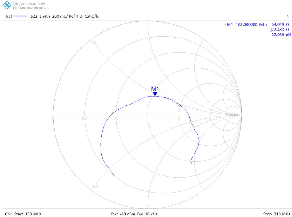
**Figure 14** Smith illustration of impedance measurement at one of the antenna ports, with antenna rods and with matching components mounted on the other ports. Also, the full system installed on a 6U structure for more realistic results.
