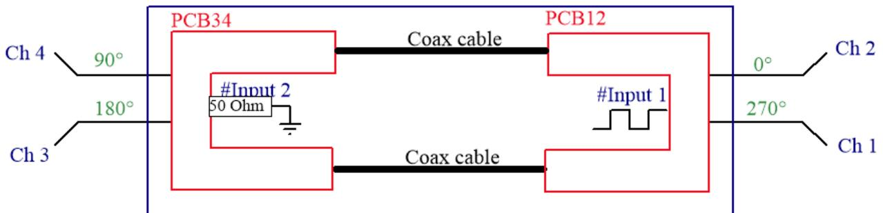
Figure 4 6U structure from the top, 2U side. Input signal at Input 2 and detection at Ch2, Ch1, Ch3 and Ch4. Green number are the expected phase of the received signal in degree at each channel. Each channel corresponds to an antenna rod.
