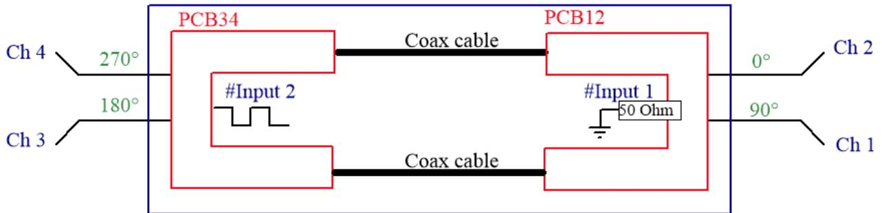
Figure 3 6U structure from the top, 2U side. Input signal at Input 1 and detection at Ch2, Ch1, Ch3 and Ch4. Green number are the expected phase of the received signal in degree at each channel. Each channel corresponds to an antenna rod.
