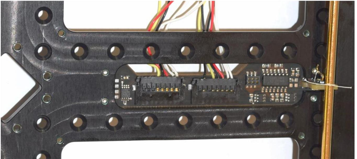
Top side with an antenna tied to the release mechanism and harnesses connected to show how the wires exit.
