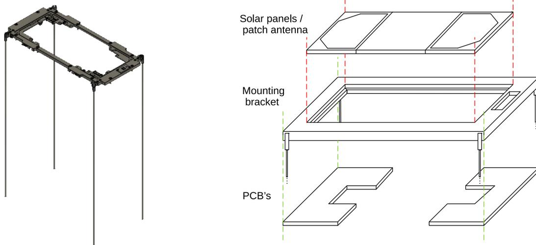
ANT-6F VHF is made of three layers screwed (with helicoils) together:
