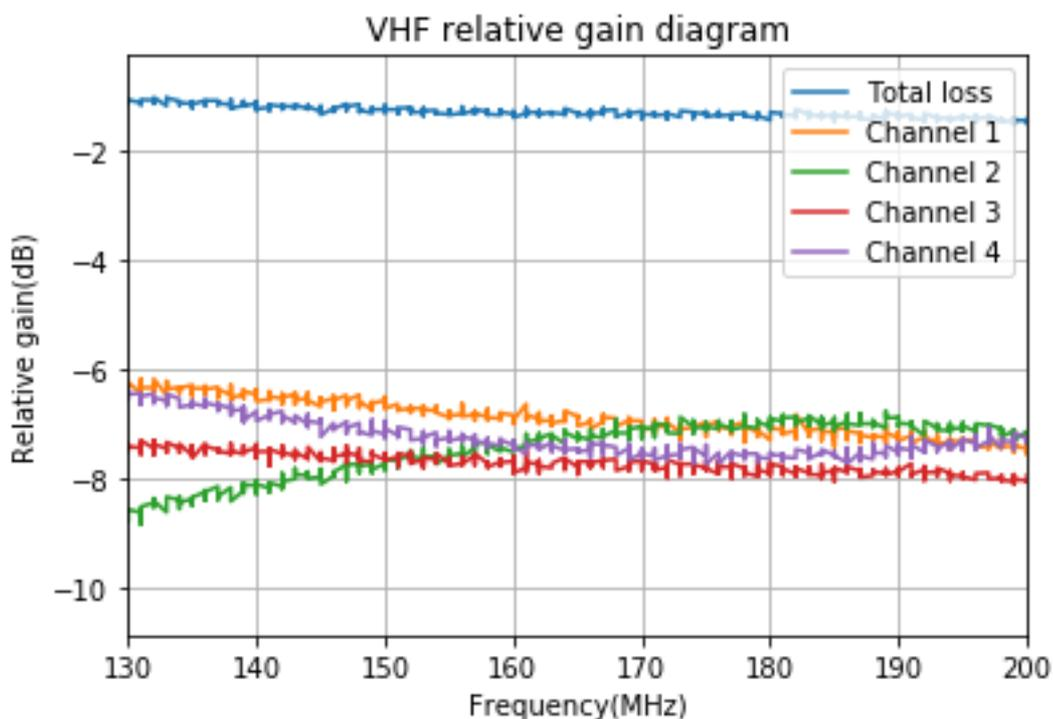
**Figure 9** Signal has been sent at Input 1 and each color corresponds to the measured signal at different channels / U.FL antenna connectors. This is the measured gain due to the PCBs and coax cables.
