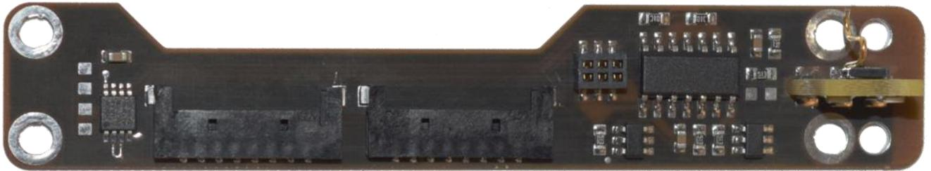
Components from left to right. I<sup>2</sup>C isolator, 2x Molex connectors, MCU connector, the MCU and the antenna release system.
