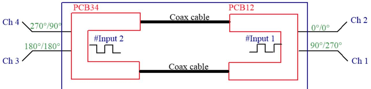
Figure 5 6U structure from the top, 2U side. Input signal at Input 1 or Input 2 and detection at Ch2, Ch1, Ch3 and Ch4. Green number are the expected phase of the received signal in degree at each channel. Each channel corresponds to an antenna rod.
