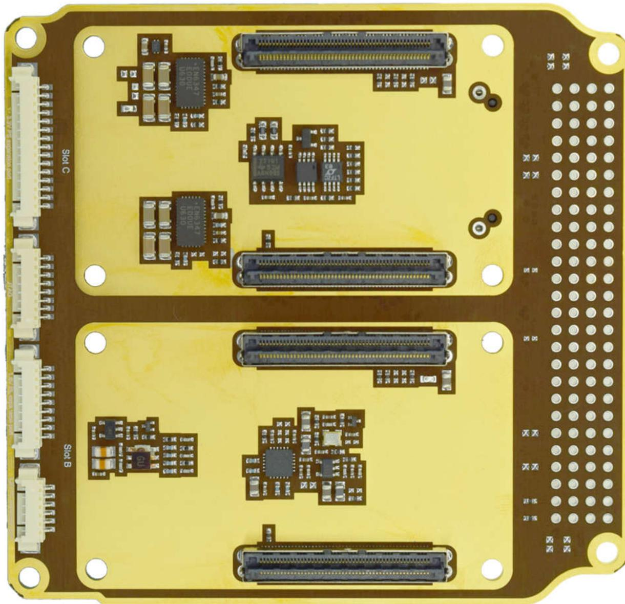
In the top gold islands are the PSU (the two left most) and the CAN and I<sup>2</sup>C isolator in the middle. In the bottom island mid is the clock fanout buffer.
