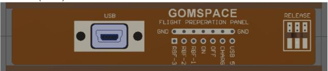
On the inside, a 12-pin horizontal PicoBlade connector allows direct interfacing to the GomSpace NanoHub (or a different subsystem). On the NanoHub the connections are then distributed to the the other systems as necessary like the kill switch to the NanoPower and the USB to the USB2serial converter on NanoHub which provides serial connection to different subsystems.
