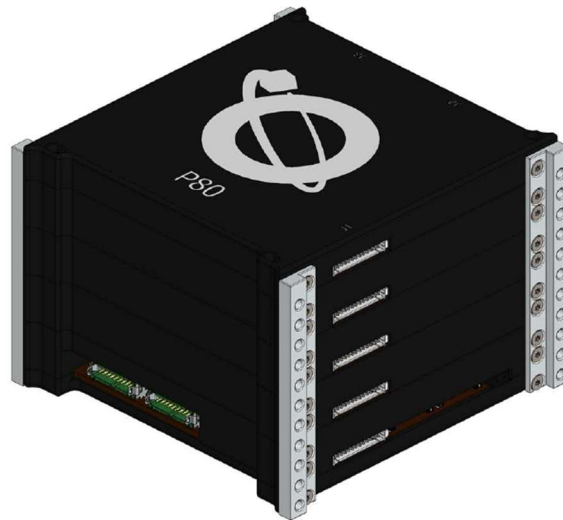
Figure 1.1: The NanoPower P80 4ACU with a single PMU and 4 ACUs.
