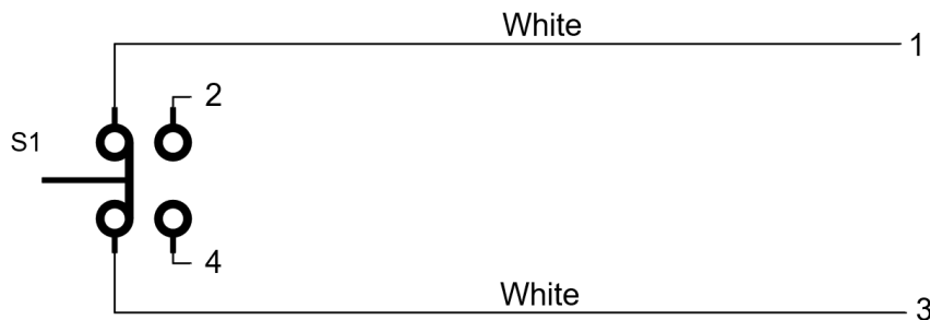
Killswitch standard configuration (NC)
