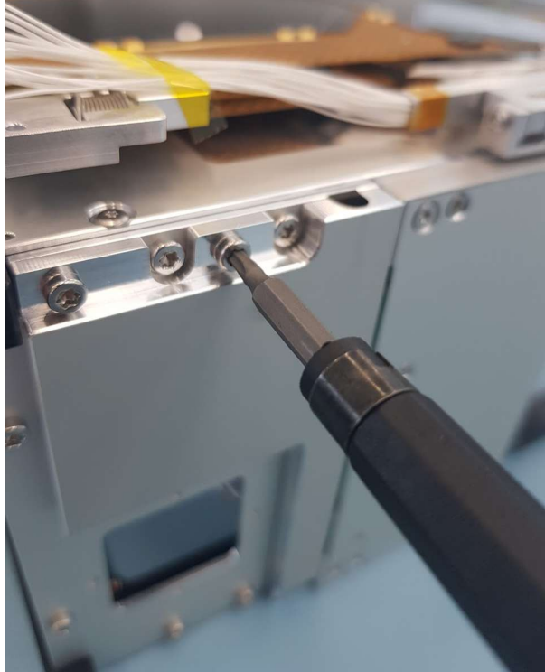
Figure 9-13: Z bracket cover part being dismantled.
