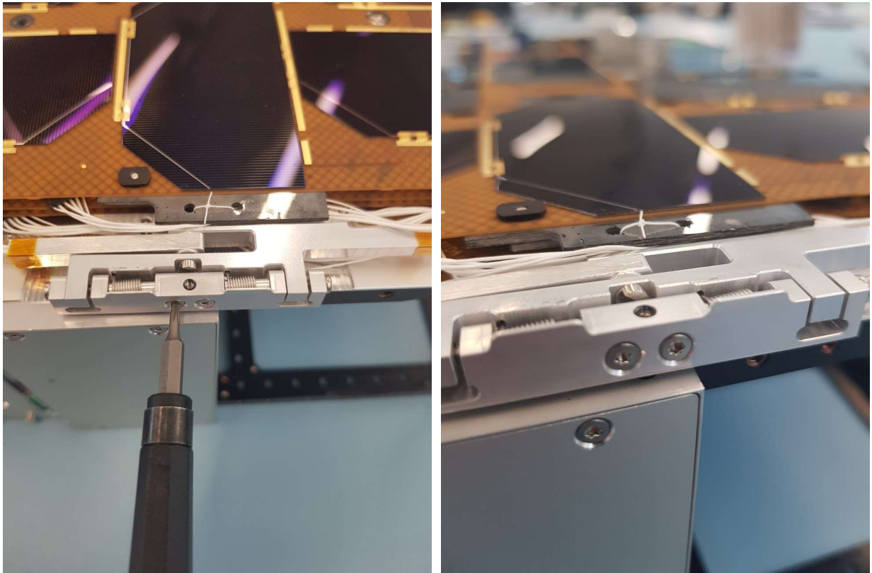
Figure 9-12: Solar array Correctly mounted onto the Output shaft and clamped from the screw interface.
