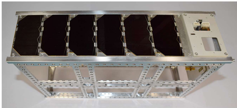
Figure 3 MSP-FPP (without GPS antenna and FSS) and NanoPower MSP (6 cell) mounted on the 3U side of a 6U structure
