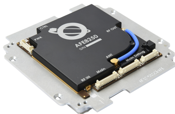
Figure 2.4: NanoCom ANT8250 with AFE8250 RF front-end
